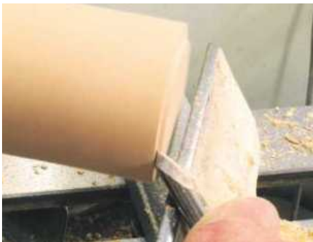
▲ Pic.12 The spindle gouge excels in cleaning across end-grain. As you can see, the bevel is at the angle of the cut I want to make
